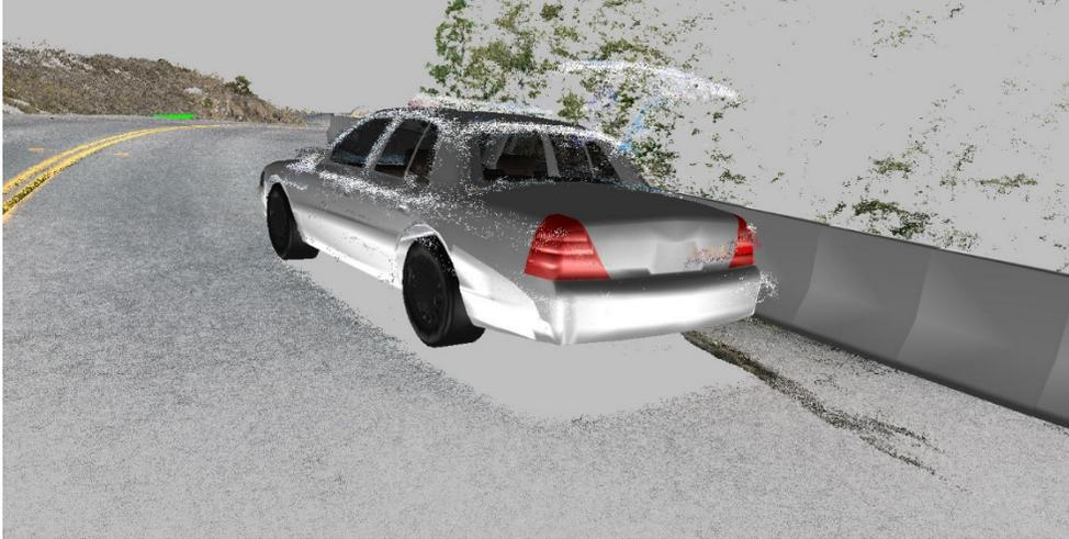
Figure 7: Accurate fitting of shape-correct car model to the generated 3D point cloud.
