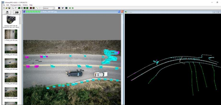
Figure 2: Feature extraction within iWitnessPRO-Agilis.
