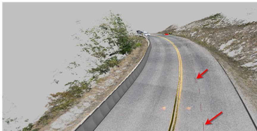
Figure 4: Feature tracing within the dense point cloud generated by iWitnessPRO-Agilis
