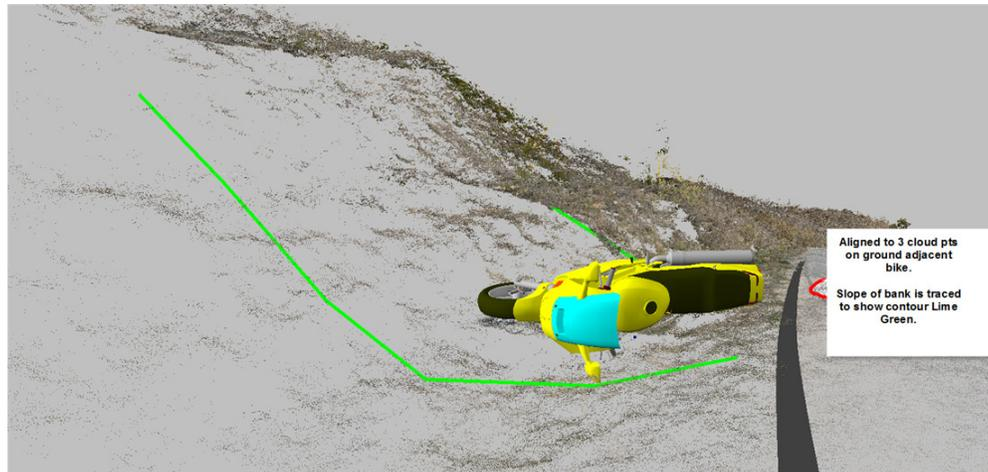
Figure 5: Motorcycle CAD symbol, inserted in the 3D point cloud.
