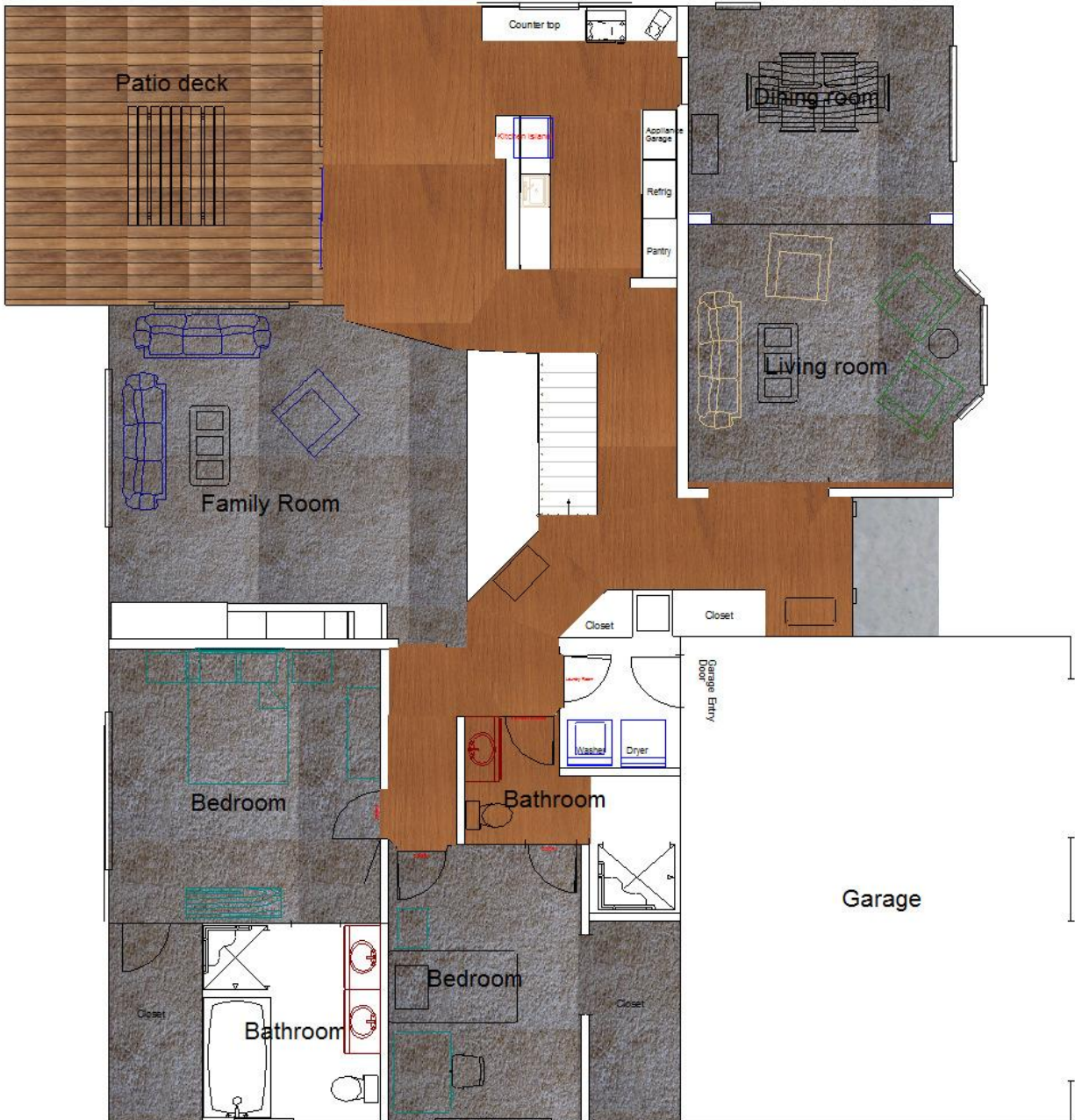
Figure 6 – Photogrammetry and Laser Range Finder measurements illustrated in CAD - Upper Level Plan View
