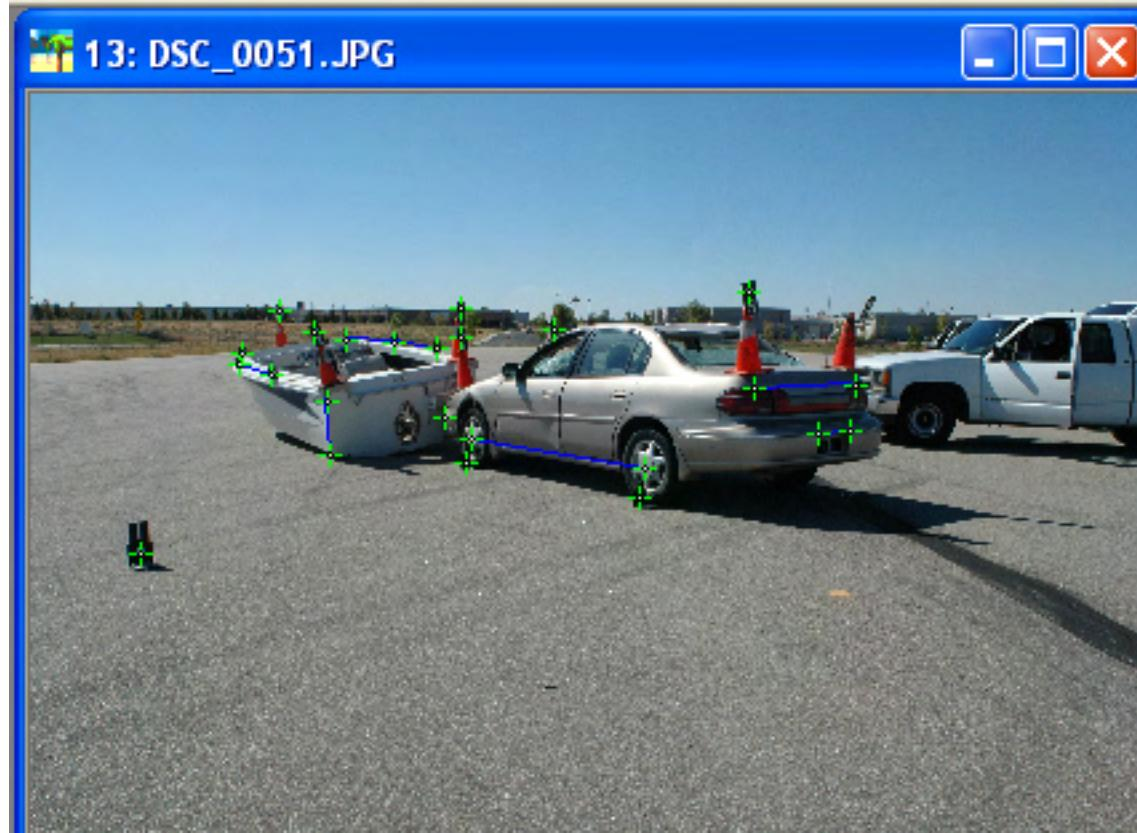
The boat disengaged the trailer from bullet vehicle impact and rode on top of the bullet car for about 150', and then slide off the car's roof, to it's final rest position as noted above.
