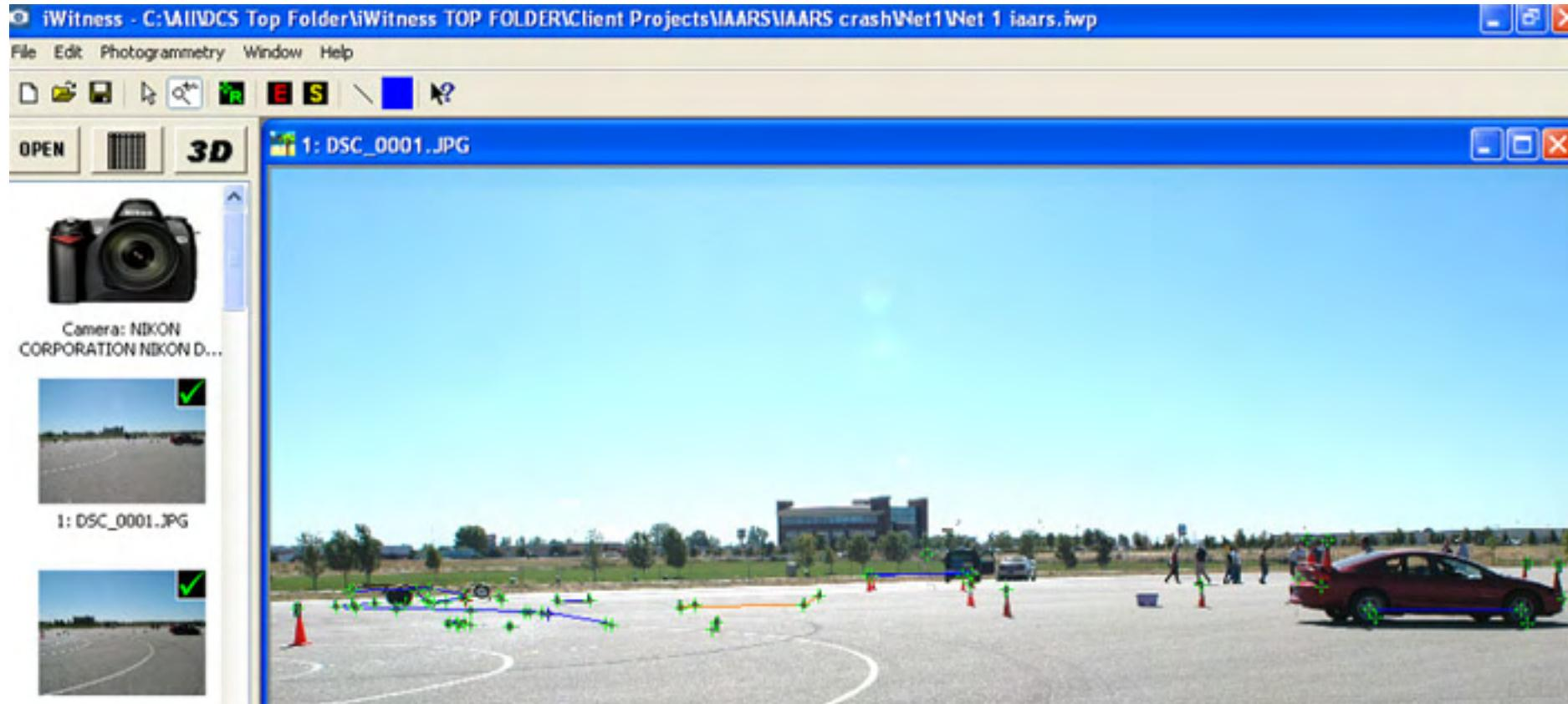
Scene overview of post collision. Bullet car #2 center, #1 tow car on right, boat trailer and crash evidence on left. iWitness 3D point marking illustrated with lime green "+" marks.
