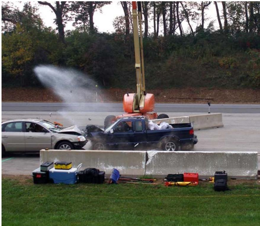
The mapping technologies used for the crash evidence collection were lasers scanners, a total station and close-range photogrammetry (digital camera and software.) The photogrammetry system used was **iWitness™**, [www.iwitnessphoto.com](http://www.iwitnessphoto.com).
