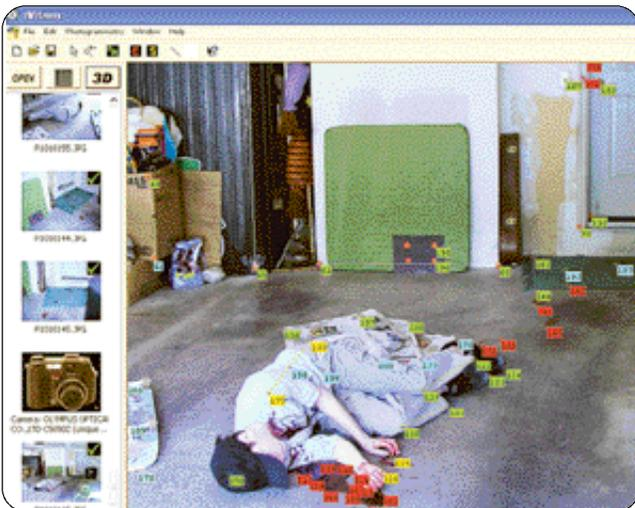
The iWitness software program was designed to facilitate diagramming of complex crime scenes from information provided in photographs. In this computer screen-capture, you can see the non-contact 3-D object points (the tiny color squares) of the murder victim and surrounding evidence.
