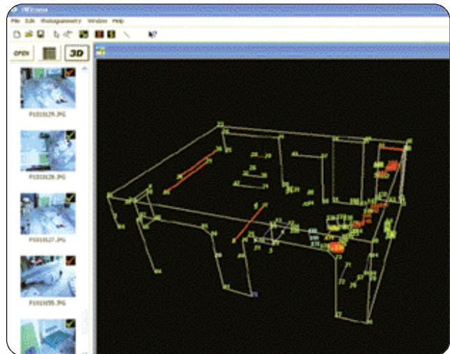
The data from the photo on the left was taken into the iWitness software to provide a 3-D graphics view of the points and lines that make up the crime scene. As you can see, all salient information is present, ready to be exported to a CAD diagramming package.
