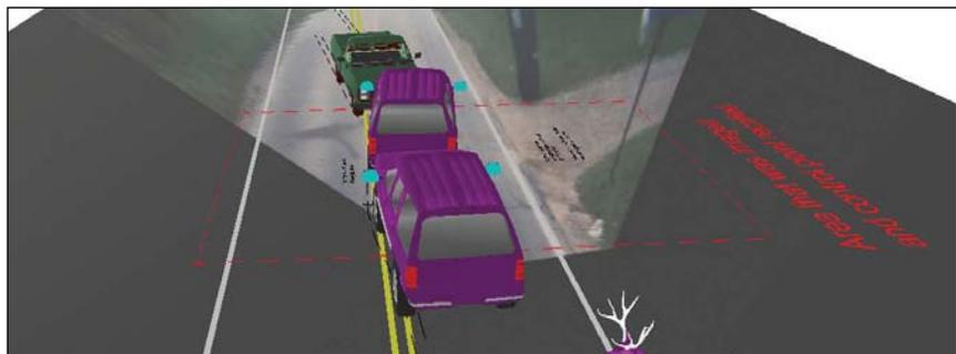
**Figure 3**—This oblique view with a CAD overlay shows how the scene may have looked just prior to and at the moment of impact. Vehicle 1 is shown here in purple; Vehicle 2 is green. The deer location is not exact and included for illustrative purposes only.
